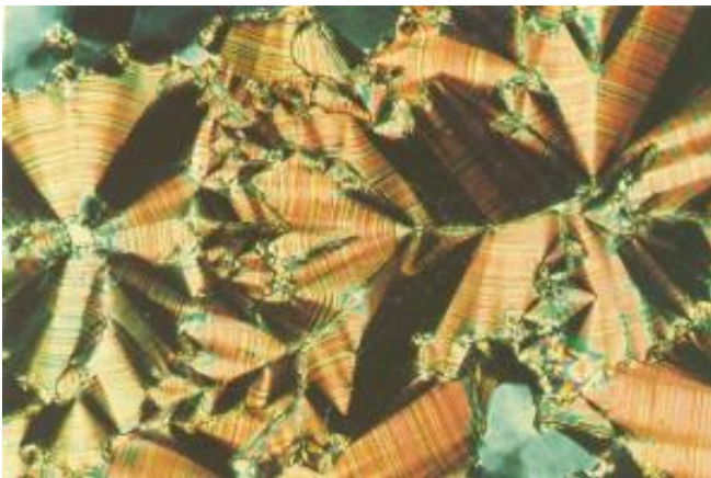
Focal conic texture of a smectic liquid crystal seen between crossed polarisers
